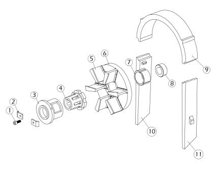
The impeller (4) is placed in the center of the blast wheel (5+6). The impeller feeds dosed quantities of abrasive onto the blades (5) of the turning blast wheel.
