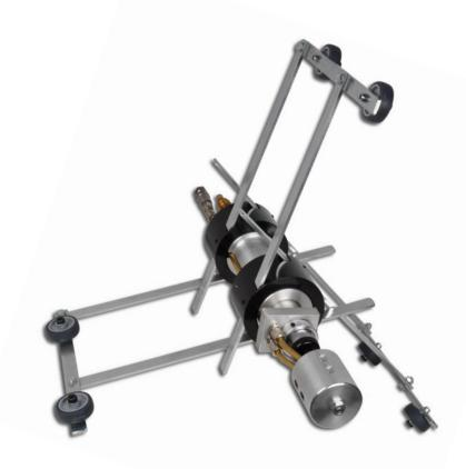
PIPECOATER-III tools are designed to coat the inside of pipe or tubing without the need to rotate pipe or tubing and to apply an even paint film thickness throughout. Generally, any type of coating may be used in this tool that can be airless sprayed. To obtain the best possible production, one man should operate the Control Gun while another man pulls the tool through the pipe or tubing.
