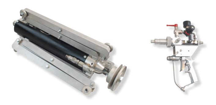
PIPECOATER-II tool is designed to coat the inside of pipe or tubing without the need to rotate pipe or tubing and to apply an even paint film thickness throughout. Generally, any type of coating may be used in this tool that can be airless sprayed. To obtain the best possible production, one man should operate the Control Gun while another man pulls the tool through the pipe or tubing.
