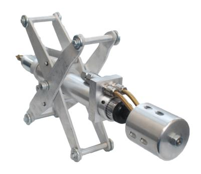
PIPECOATER-III tools are designed to coat the inside of pipe or tubing without the need to rotate pipe or tubing and to apply an even paint film thickness throughout. Generally, any type of coating may be used in this tool that can be airless sprayed. To obtain the best possible production, one man should operate the Control Gun while another man pulls the tool through the pipe or tubing.
