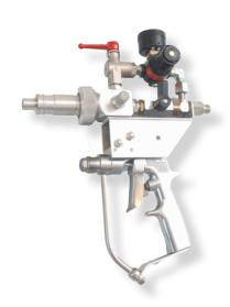
PIPECOATER-I tools is designed to coat the inside of pipe or tubing without the need to rotate pipe or tubing and to apply an even paint film thickness throughout. Generally, any type of coating may be used in this tool that can be airless sprayed. To obtain the best possible production, one man should operate the Control Gun while another man pulls the tool through the pipe or tubing.
