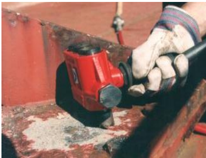
Rust removal on ships deck using 153.5300 triple head scaler
